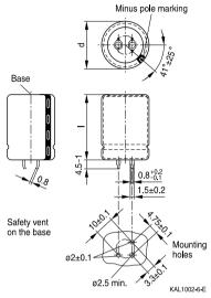
Snap-in capacitors are also available with 3 terminals (length (4.5-1) mm). PET insulation is marked with label "PET" on the sleeve.
